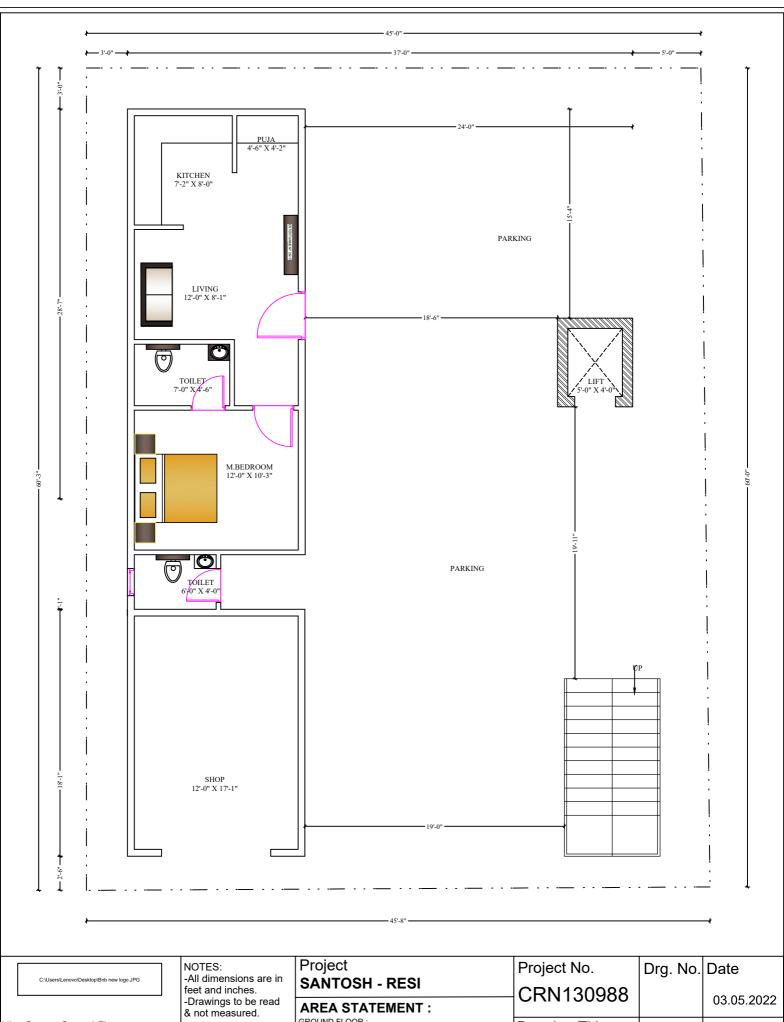
GROUND FLOOR: 1BHK, Staircase & Clinic room: 778.59 sq.ft Parking: 1277.25 sq.ft Lift: 35.75 sq.ft Hive Space, Ground Floor, **Drawing Title** Scale Details will supercede Ramalayam rd, GROUND W**→**E Laxmi Cyber city, all drawings. NTS FLOOR R2 Kondapúr, \$ Hyderabad, Telangana 500084 Architect: Rohini Chakravarthy
